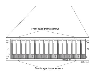
Figure 86. Front cage frame screw locations
